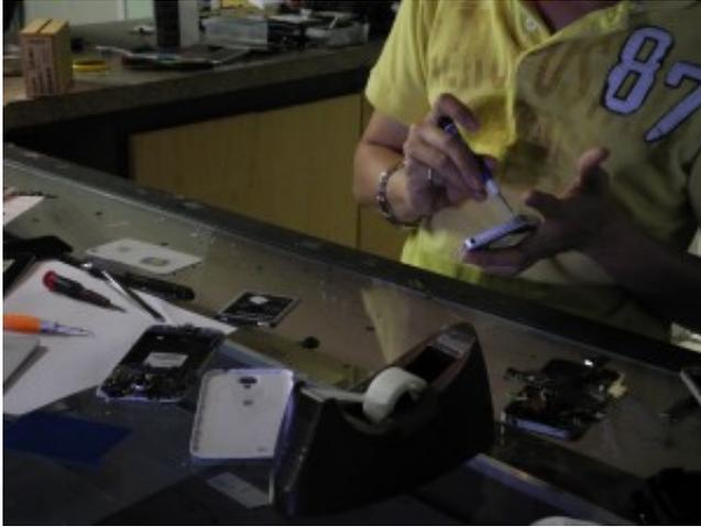
Figure 2: Cell phone repair technician replaces iPhone 4 cracked screen on countertop in front of customers. (Photo Credit: Briel Kobak)
